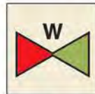
Fire main section valve
