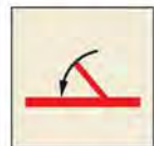
'A' Class self-closing fire door 6760 EE, GG & JJ
