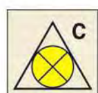
Remote vent. shut-off for cargo spaces 6780 EE, GG & JJ
