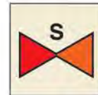
Sprinkler section valve
