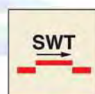
'A' Class semi-watertight self-closing sliding fire door 6774 EE, GG & JJ
