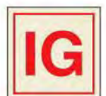
Inert gas installation
