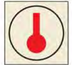
Space monitored by heat detector(s) 6874 EE, GG & JJ
