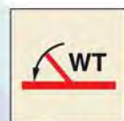
'A' Class self-closing watertight fire door 6761 EE, GG & JJ
