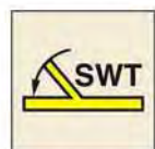
'B' Class self-closing semi-watertight fire door 6765 EE, GG & JJ
