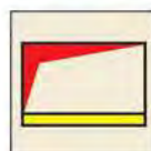
High expansion foam supply tank
