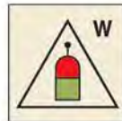
Remote release station for water
