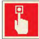
Manually operated call point 6872 EE, GG & JJ
