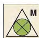
Remote vent. shut-off for machinery spaces 6779 EE, GG & JJ
