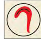
Space monitored by smoke detector(s) 6873 EE, GG & JJ
